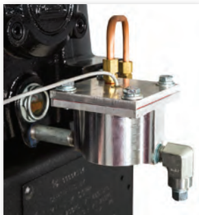
Low oil sensor does not allow unit to start when oil levels fall below an adequate level
